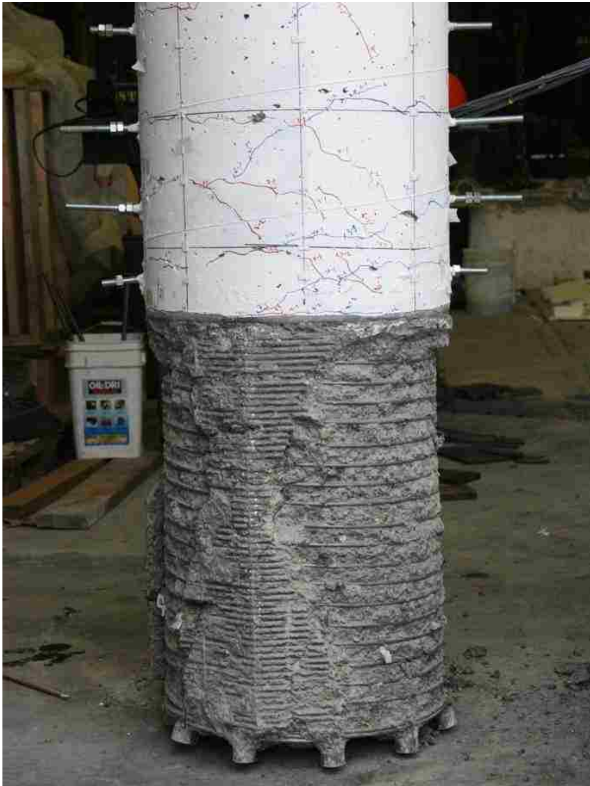
Figure C-0-13. DS-2 – Column damage after cyclic testing
